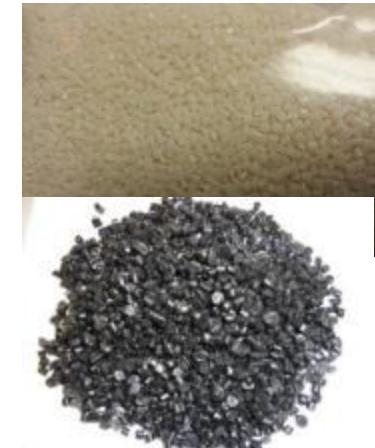
Pellets that have been made from polymer separated and purity enhanced Recycled Plastic
